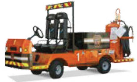
Bigfoot with SBCA seats, rear platform holds two Amerex units, battery roll-out box and light bar.
