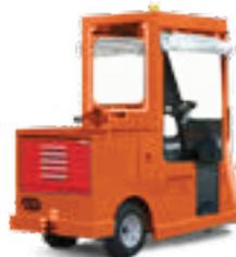
MX-600 mobile maintenance vehicle with cab, clear vinyl enclosure and strobe light.
