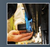
6. Line the bumper up with the front of the Blue Guardian and insert the bolts into the front of the bumper with the washer at the head of the bolt and the split washer between the Blue Guardian and the back plate.
