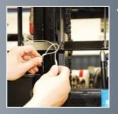
4. Raise the tines to a working height and slip leash around the carriage and through the loop. If there is enough length wind the leash around the carriage one more time. Then thread this through bottom of backrest.
