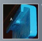
Clean channel and center notch of the forklift carriage. Make sure it is clear of wood splinters and other debris.
