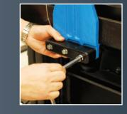
7. Holding the back plate in place, tighten all 3 bolts from the front side of the Blue Guardian.
