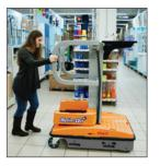
Very light overall weight of the unit ONLY 280 Kg makes it easy and comfortable to be pushed around and able to be used on every floor, even mezzanine floor.
