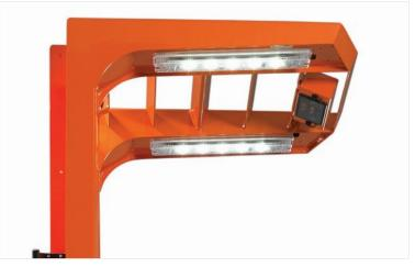
Overhead guard with integral LED working lights
