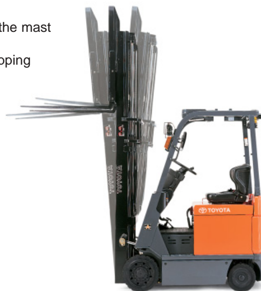
The Active Mast Function Controller controls the mast tilt angle and speed, depending on the weight and height of the load.
